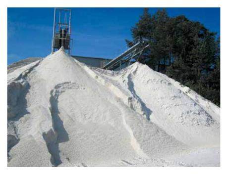
Figure 10: Feldspar raw material requires processing before introduction to the market. Customers are supplied with milled feldspar of different mesh sizes (Photo: BGR).
