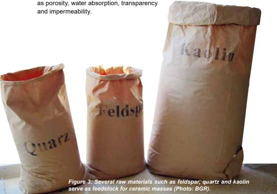
For the production of ceramic masses (Figure 4), which are a mixture of raw materials, as well as in **glazes** and in **enamel** mainly soda and potash feld-spars are used. "Impure" feldspars that contain both endmembers are also valuable because of their aluminium content. It reduces tension in the crystal lattice and thus reduces fire cracks and improves evenness, chemical durability and rupture strength of the final product.
