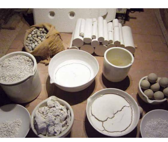
Figure: 4: Before application in the final stage, feldspar raw material passes through various intermediate processing steps from filter cake to ceramic masses (Photo: BGR).
