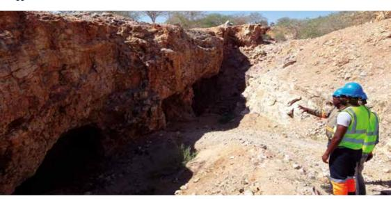
Figure 16: Remnants of room and pillar mining at historic mine site at Rubicon pegmatite (Photo: BGR-GSN-Project 2019, with kind permission of Lepidico Chemicals Namibia (Pty) Ltd.).
