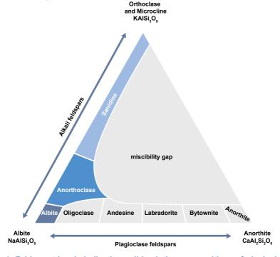
Figure 1: Feldspar triangle indicating solid solution compositions of plagioclases and alkali feldspars feldspars (after DEER et al. 1992).
